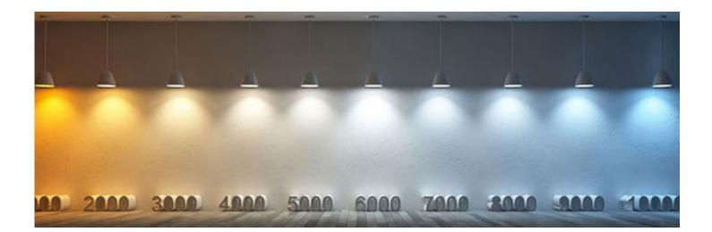
So what is color temperature anyway? As a review, color temperature (Correlated Color Temperature, or CCT, in lighting tech jargon) is essentially a gauge of how yellow or blue the color of light emitted from a light bulb appears. It's measured in the Kelvin unit and is most commonly found between 2200 Kelvin degrees and 6500 Kelvin degrees.
